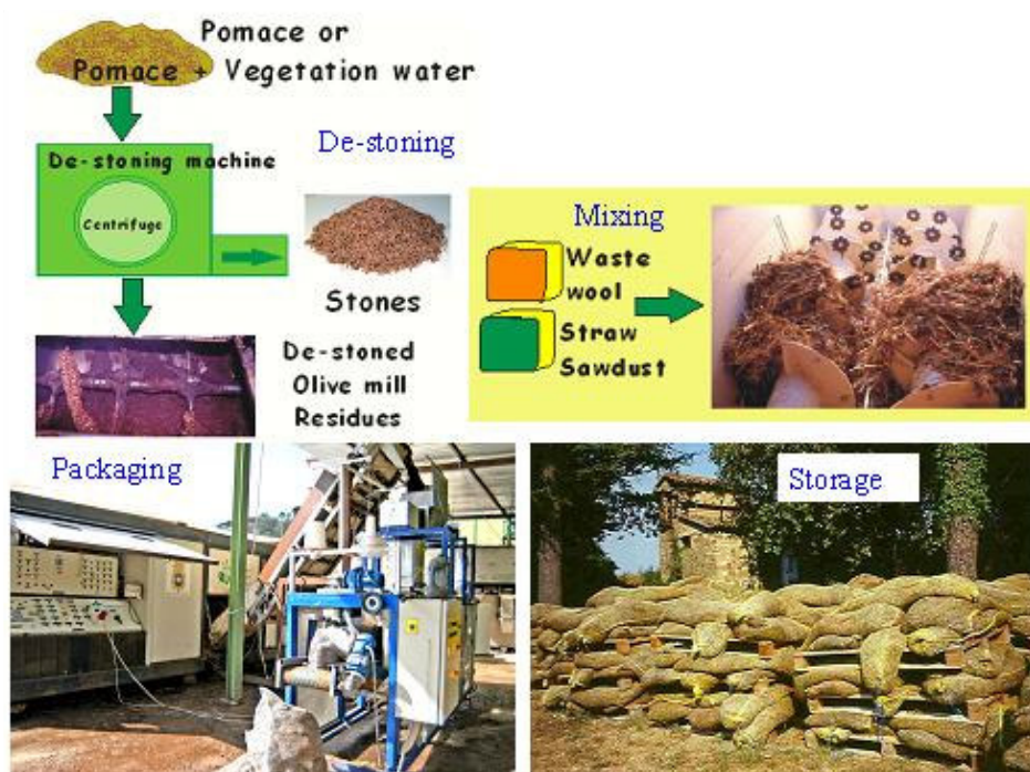
Figure 1. Diagram of the M.A.T.Re.F.O. procedure
